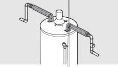
Typical horizontal piping arrangement
